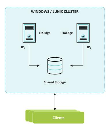
FIXEdge supports work in multiple node clusters with state replication, failover and recovery functionalities. FIXEdge clusters are based on the RedHat 6/7 pacemaker with corosync and are used in production in some of the most demanding environments in the world.
