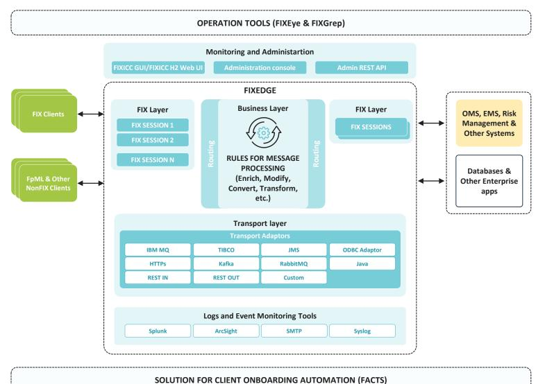
Client applications communicate with FIXEdge via one of multiple supported message protocols (e.g. JMS, IBM MQ,REST) employing FIXEdge transport adaptors.
