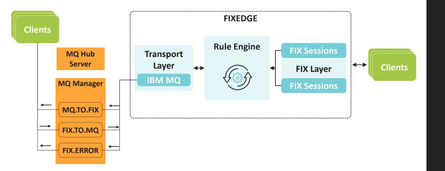
IBM MQ Transport Adaptor is an add-in for FIXEdge that allows clients to communicate with FIXEdge over IBM MQSeries middleware.
