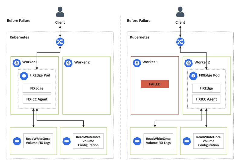
FIXEdge can be deployed in containerized environments like Kubernetes to leverage HA facilities and flexible workload distribution for multiple applications across servers.
