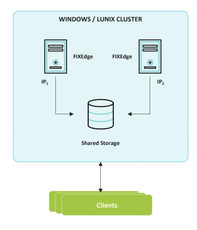
FIXEdge supports work in multiple node clusters with state replication, failover and recovery functionalities. FIXEdge clusters are based on the RedHat 7/8 pacemaker with corosync and are used in production in some of the most demanding environments in the world.
