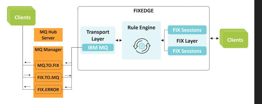
IBM MQ Transport Adaptor is an add-in for FIXEdge that allows clients to communicate with FIXEdge over IBM
