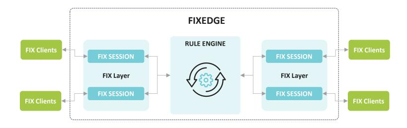
FIXEdge is mostly used as a generic smart router and a common FIX connectivity service to delegate all FIX connectivity-related tasks in the enterprise architecture.
