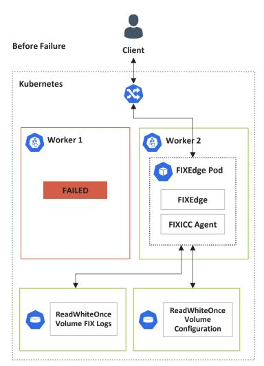
FIXEdge can be deployed in containerized environments like Kubernetes to leverage HA facilities and flexible workload distribution for multiple applications across servers.
